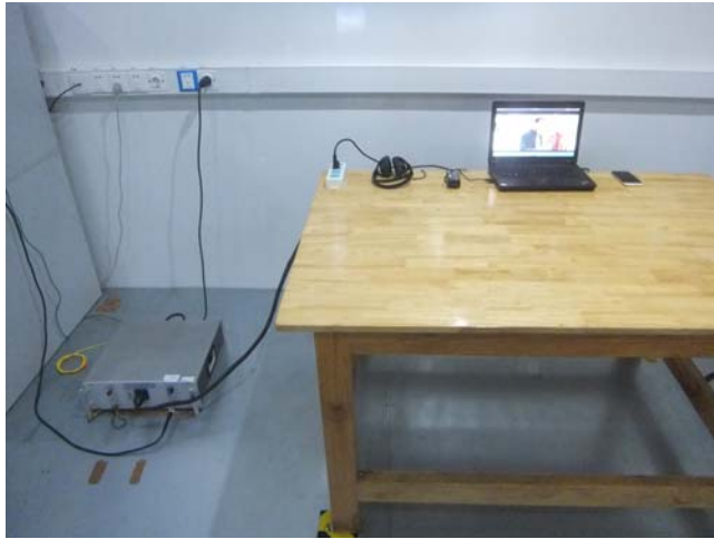
Conducted Emissions Test Setup – Front View
