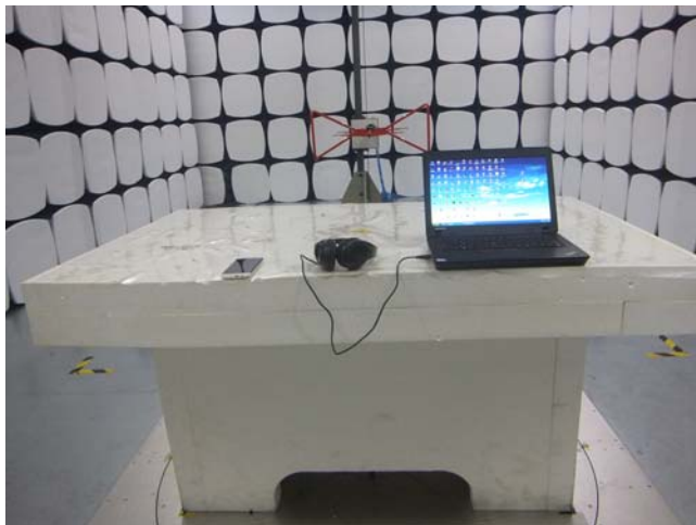
Radiated Spurious Emissions Test Setup Below 1GHz
