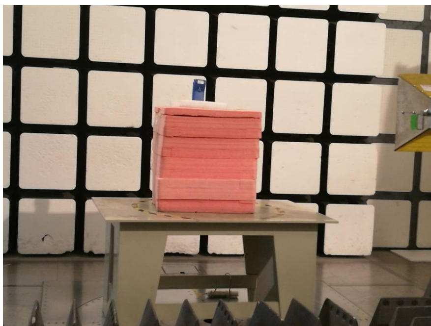
Radiated Emissions View (Above 1 GHz)
