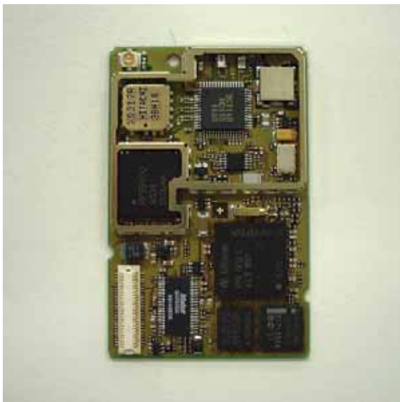
MC46 Module Interior View
