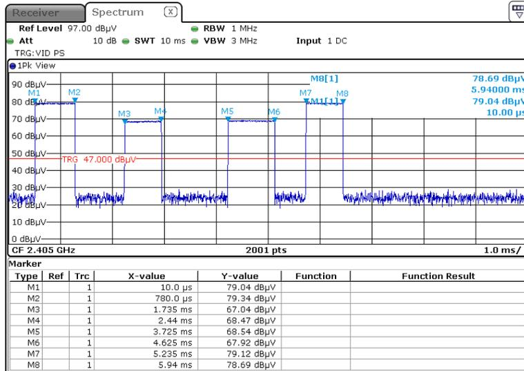
Note: The markers M1, M2, M7 and M8 are marker values according to the response of the companion device. The markers M3, M4, M5 and M6 represent the on-time of the EUT.
