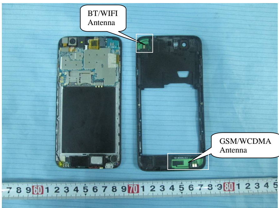
EUT – Bare Cover off View
