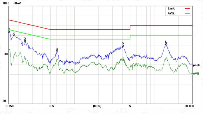
Line Conducted Emission Test Line 2-N
