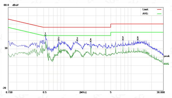
Line Conducted Emission Test Line 1-L
