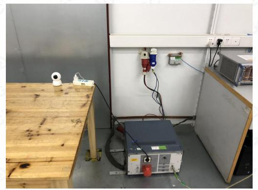
CONDUCTED EMISSION TEST SETUP
