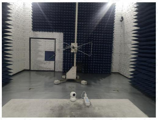
FCC RADIATED EMISSION TEST SETUP ABOVE 1GHZ
