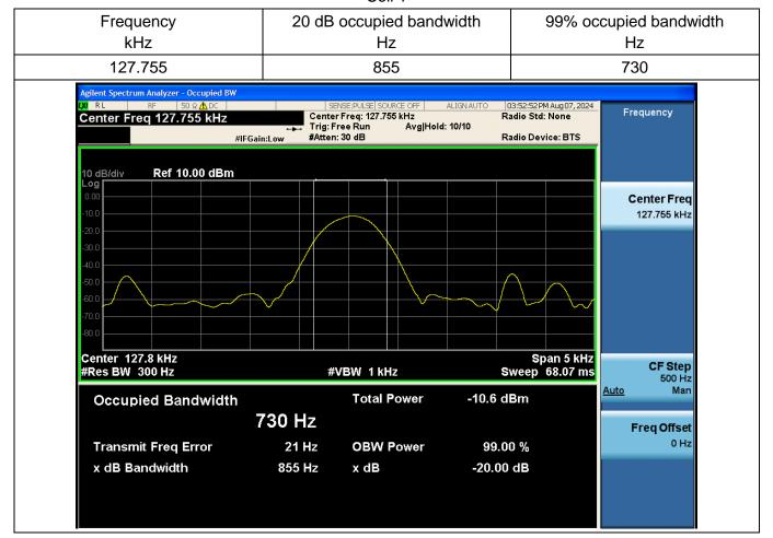
**Note:** Because the measured signal is CW-like, adjusting the RBW per C63.10 would not be practical
