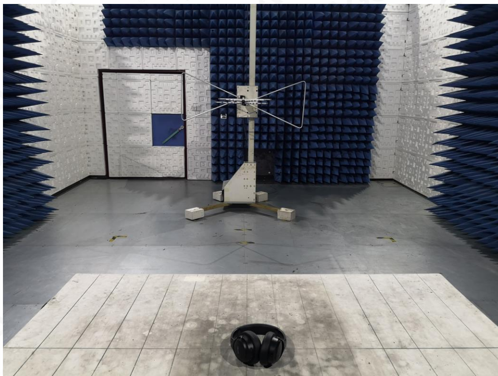
RADIATED EMISSION TEST SETUP ABOVE 1GHZ
