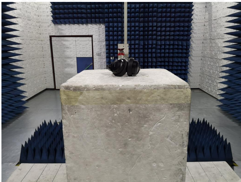
RADIATED EMISSION TEST SETUP ABOVE 1GHZ
