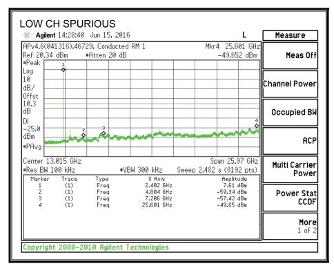
Note – Limit line should be -12.8 dBm for the Low Channel Spurious plot.
