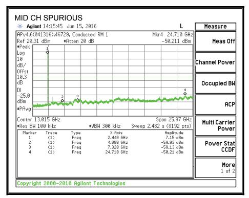
Note – Limit line should be -12.8 dBm for the Mid Channel Spurious plot.
