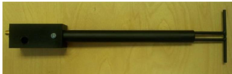
Figure 1 – MVG COMOSAR Validation Dipole
