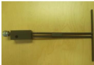
**Figure 1 – MVG COMOSAR Validation Dipole**
