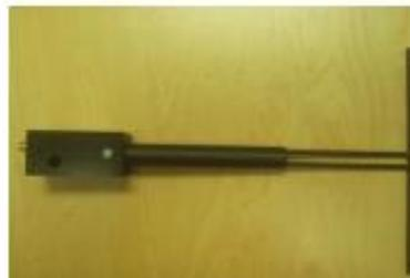
Figure 1 – MVG COMOSAR Validation Dipole
