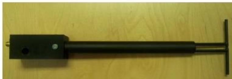
**Figure 1 – MVG COMOSAR Validation Dipole**
