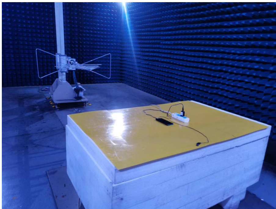
Photo of Radiated Emission Measurement (Above 1G)
