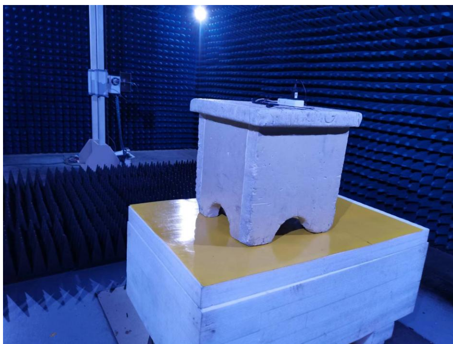
Photo of Radiated Emission Measurement (Above 1G)
