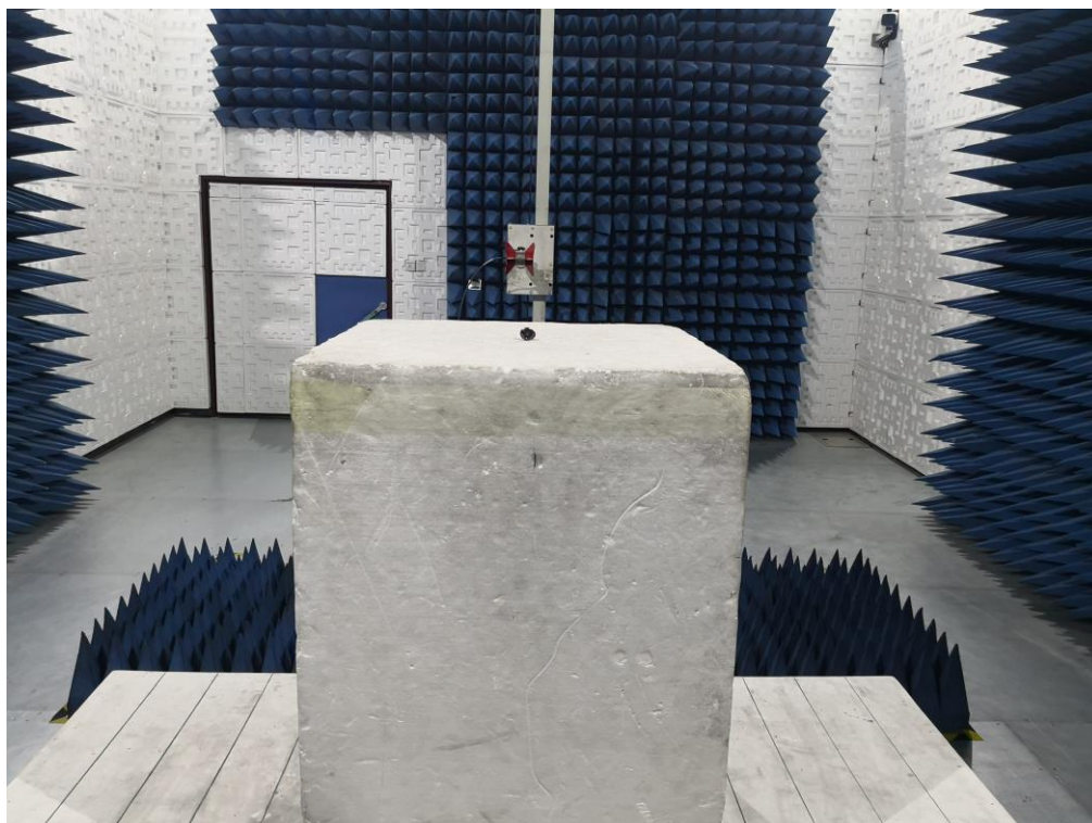
RADIATED EMISSION TEST SETUP ABOVE 1GHZ
