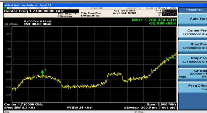
(Channel Bandwidth: 1.4 MHz)_LCH_QPSK_1RB#5
