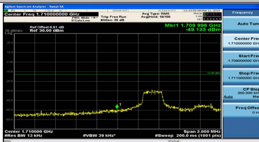
(Channel Bandwidth: 5 MHz)_LCH_QPSK_12RB#0
