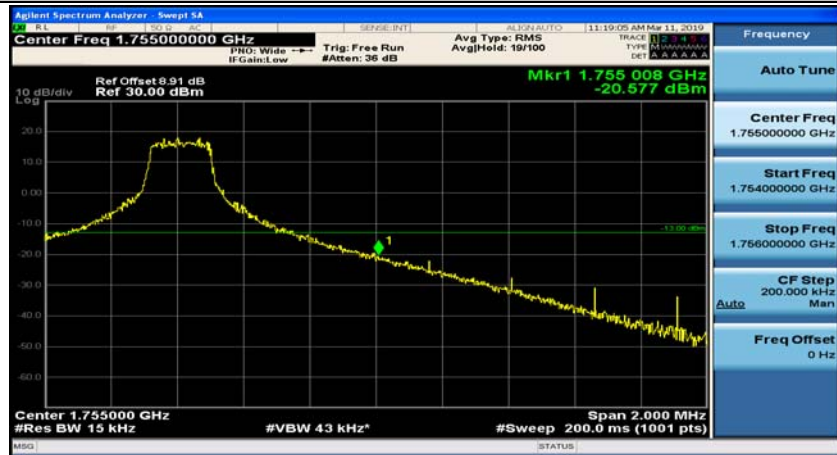
Channel Bandwidth: 10 MHz_HCH_QPSK_25RB#0
