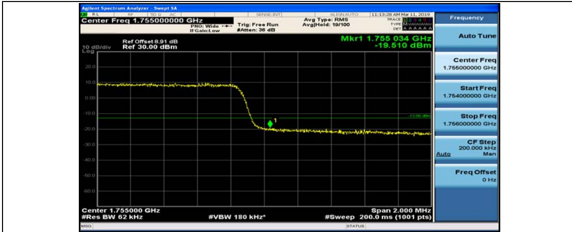
(Channel Bandwidth: 3 MHz)_LCH_16QAM_1RB#0
