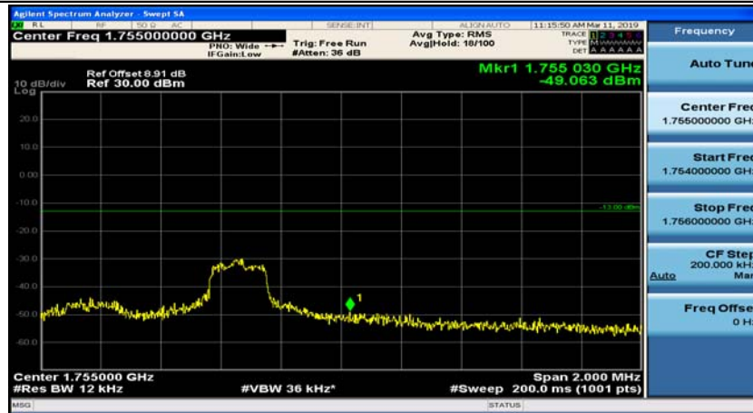
(Channel Bandwidth: 5 MHz)_HCH_16QAM_1RB#12
