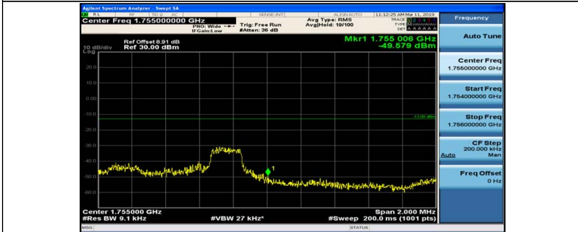
(Channel Bandwidth: 3 MHz)_HCH_16QAM_1RB#7
