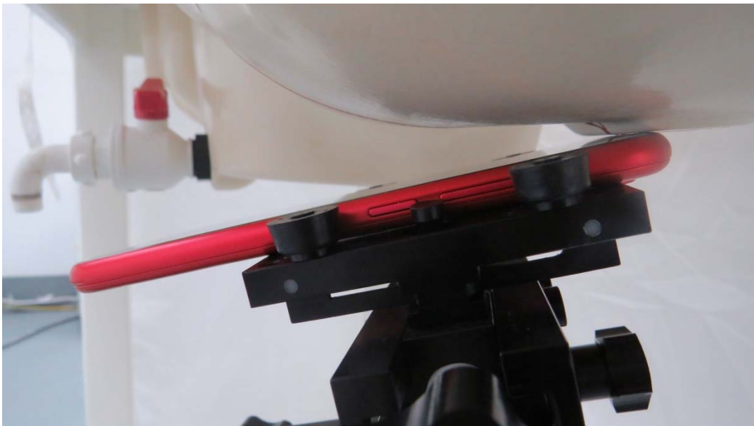
Picture 7: Left Hand Tilt 15 Degree Position
