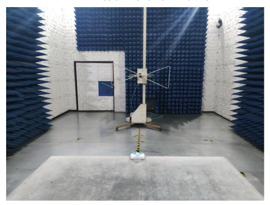
RADIATED EMISSION TEST SETUP ABOVE 1GHz
