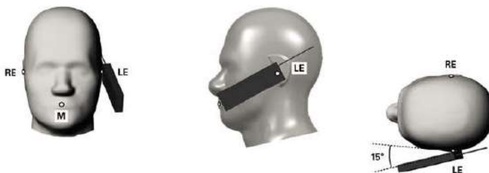
Fig.11.4 Illustration for Tilted Position
