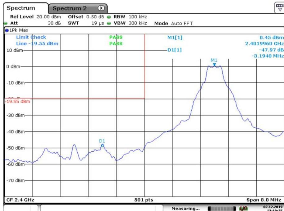
**Band Edge, Right Side**
