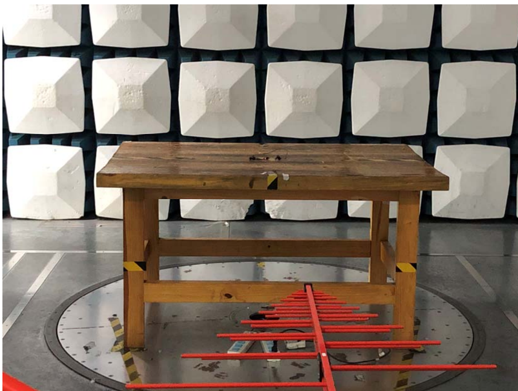
Radiated Emission Above 1GHz View
