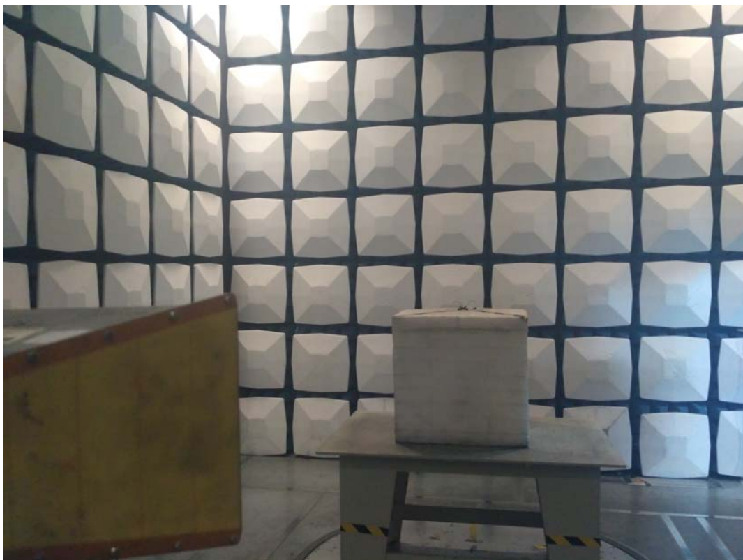
Radiated Emission Above 1GHz View
