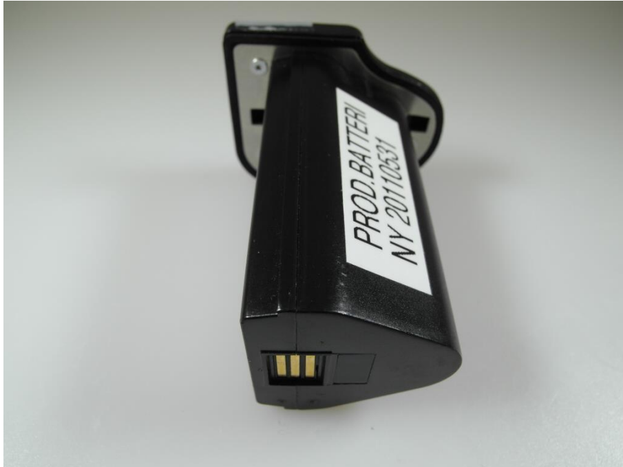
Photo 11: battery interface port
