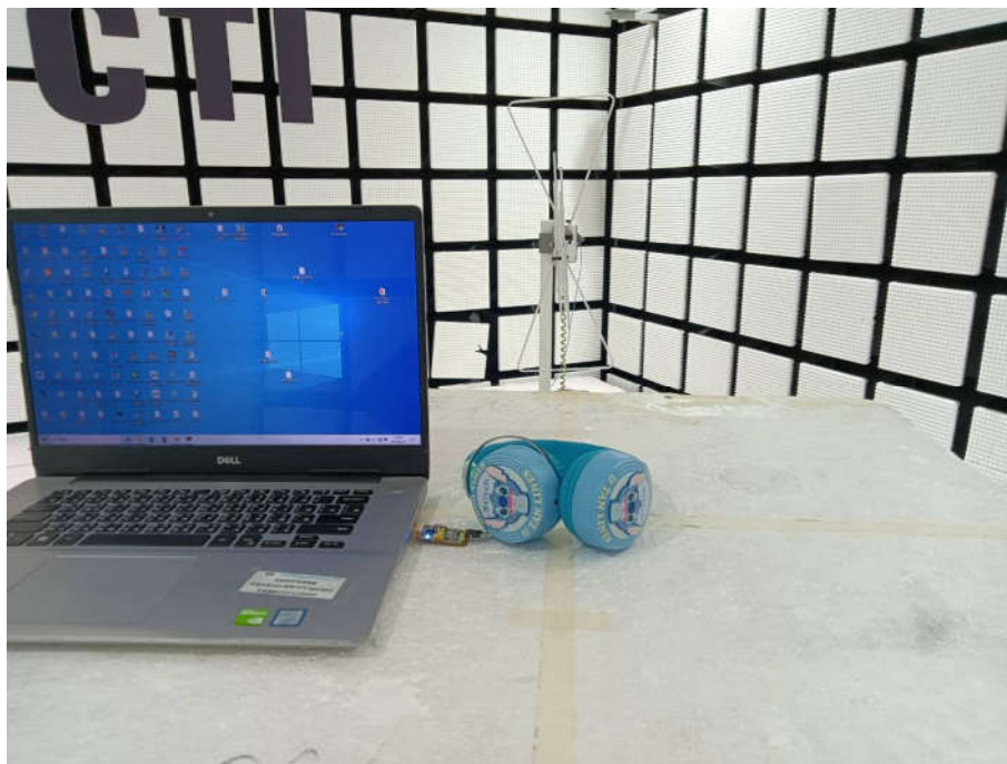
Radiated spurious emission Test Setup-1(Below 1GHz)
