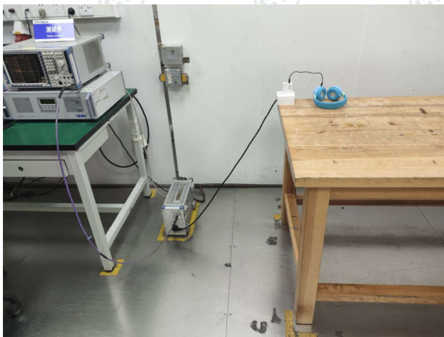
Conducted Emissions Test Setup
