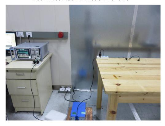
FCC RADIATED EMISSION TEST SETUP
