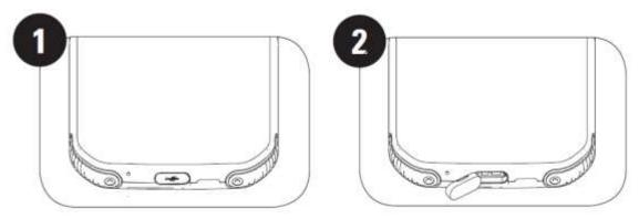
1. Connect the USB power cable to the charging power adapter.
