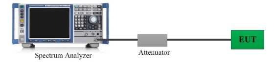
A short RF cable with low cable loss connected to the EUT antenna port, which was provided by manufacturer. The cable loss of this RF cable was offset into the setting of test equipment, which was provided by manufacturer  $\blacktriangle$ .
