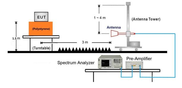
18GHz ~40GHz Test Setup:
