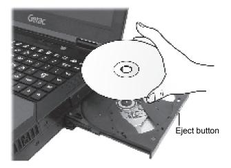
To remove a disc, hold the disc by its outer edge and lift it up from the tray.
