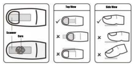
After placing your finger on the scanner, lift it up and place it down again. You should slightly move your finger between each reading. Repeat this action several times (normally between 12 and 16 times) until the fingerprint is enrolled.
