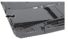
Fit another battery pack into place. With the battery pack correctly oriented, attach its connector side to the battery compartment at an angle (●) and then press down the other side (●).
