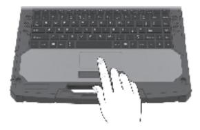
The touchpad consists of a rectangular pad (work surface) and a left and a right button. To use the touchpad, place your forefinger or thumb on the pad. The rectangular pad acts like a miniature duplicate of your display. As you slide your fingertip across the pad, the pointer (also called cursor) on the screen moves accordingly. When your finger reaches the edge of the pad, simply relocate yourself by lifting the finger and placing it on the other side of the pad.
