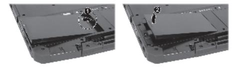
7. Slide the battery latch toward the locked position  $(\Box)$ .
