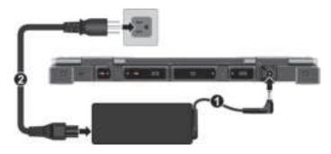
3. Power is being supplied from the electrical outlet to the AC adapter and onto your computer. Now, you are ready to turn on the computer.
