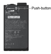
When the battery pack is not installed in the computer and you want to know the battery charge, you can press the push-button to see the number of LEDs that light up. Each LED represents 20% charge.
