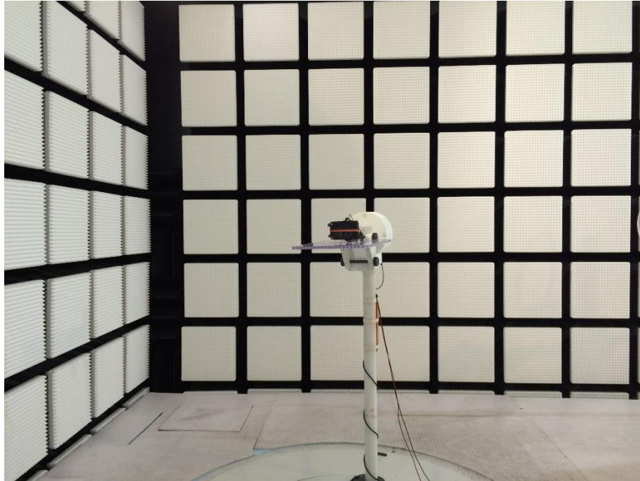
Photo 1 (RSE set-up / Fully-anechoic chamber):
