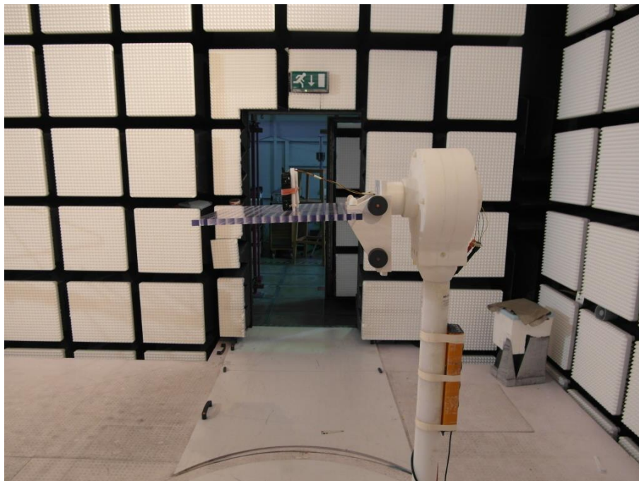
Photo 11 (RSE set-up with ID-card / Fully-anechoic chamber):
