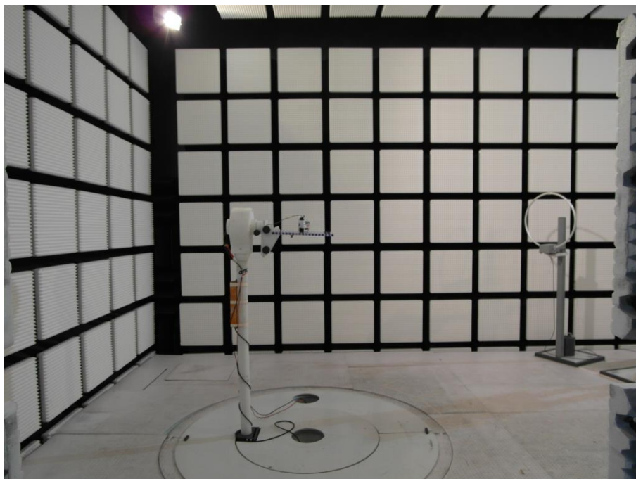
Photo 4 (RSE set-up with wireless charging unit / Fully-anechoic chamber):
