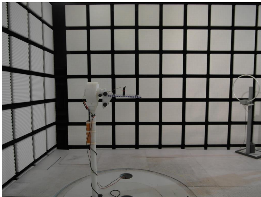
Photo 10 (RSE set-up with ID-card / Fully-anechoic chamber):
