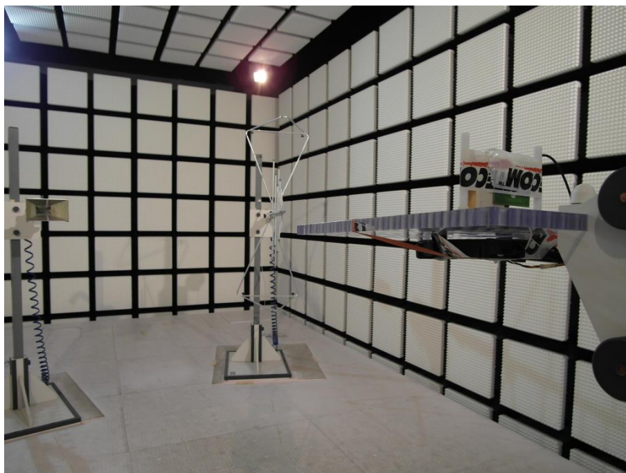
Photo 16 (RSE set-up with external antenna / Fully-anechoic chamber):
