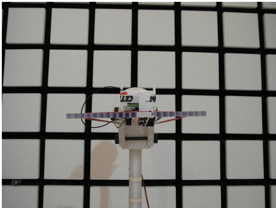
Photo 13 (RSE set-up with external antenna / Fully-anechoic chamber):
