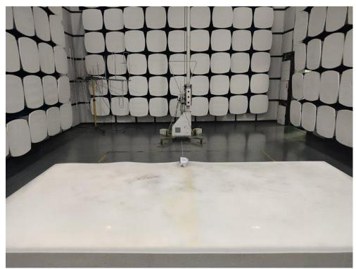
1.1. Photo of Radiated Emission test
