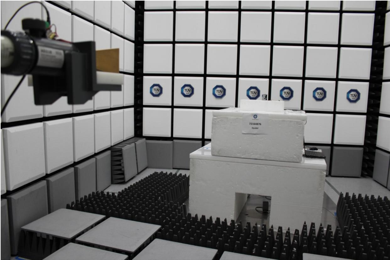
**Radiated Emissions Test Setup (Above 18GHz)**
