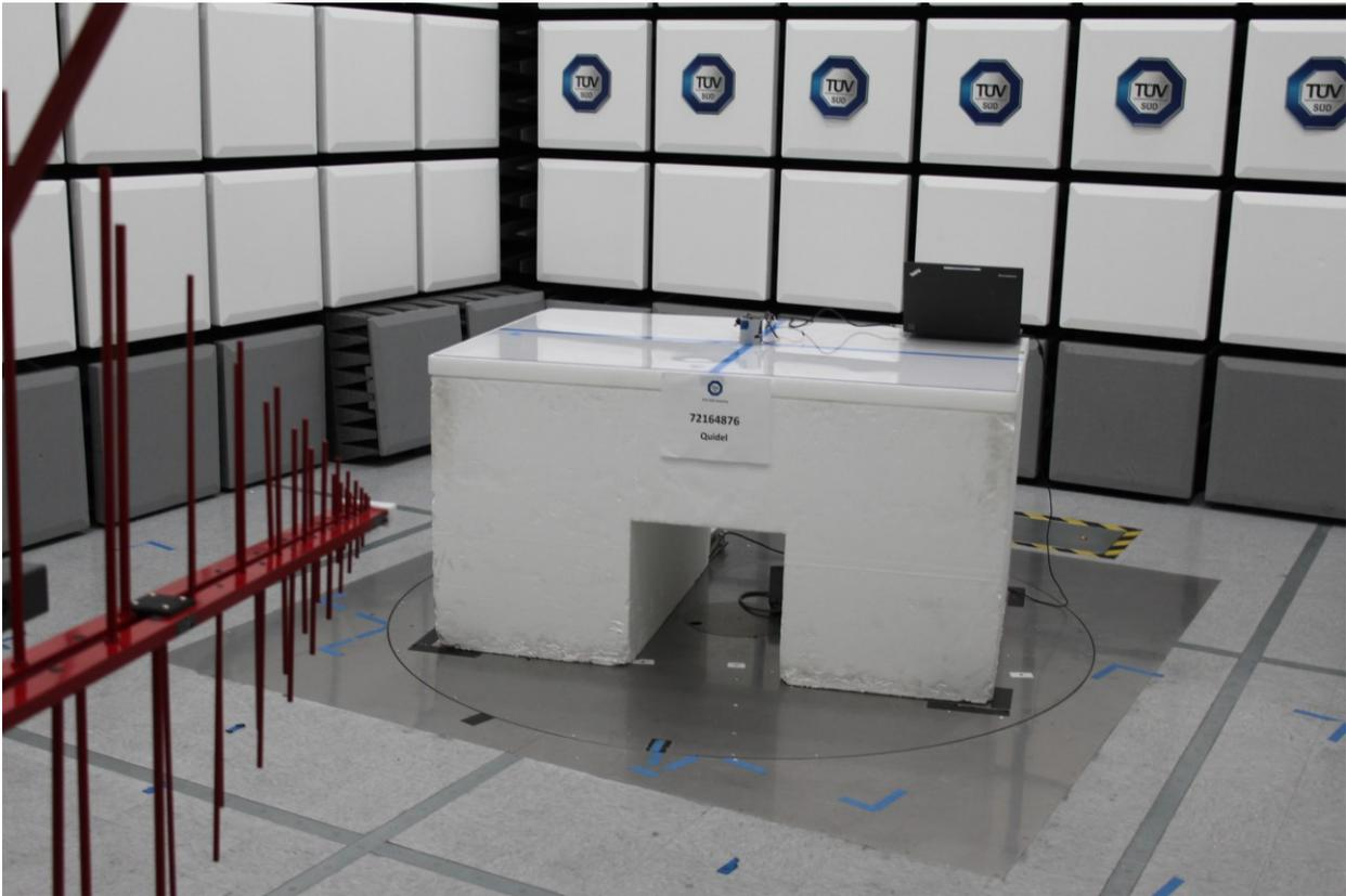
**Radiated Emissions Test Setup (30MHz to 1GHz)**
