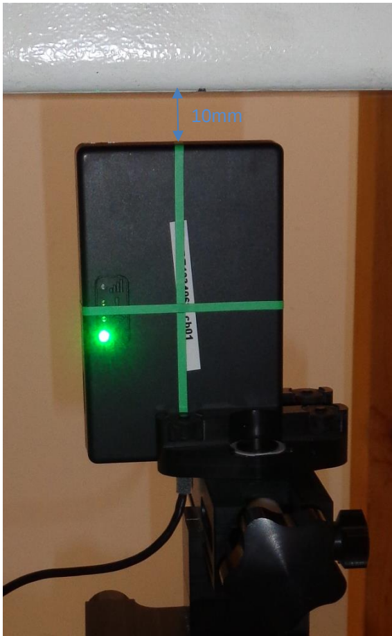
Top side of the device against the phantom with 10mm separation.
