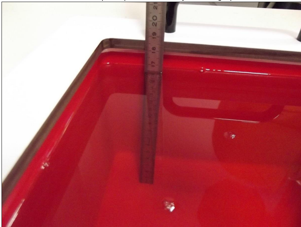
Photo 1: Liquid depth 450 MHz body simulating liquid
