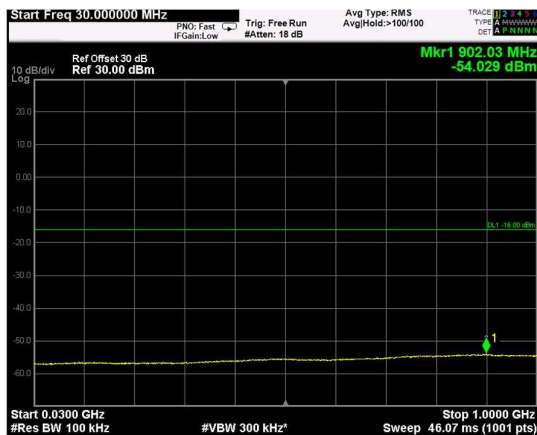
Channel: BOTTOM, Modulation: 16QAM, BW=15MHz, Range: Lower
