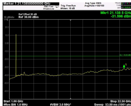
Channel: BOTTOM, Modulation: 256QAM, BW=15MHz, Range: Upper
