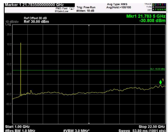
Channel: TOP, Modulation: 256QAM, BW=10MHz, Range: Upper
