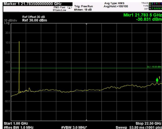
Channel: MIDDLE, Modulation: 16QAM, BW=15MHz, Range: Upper
