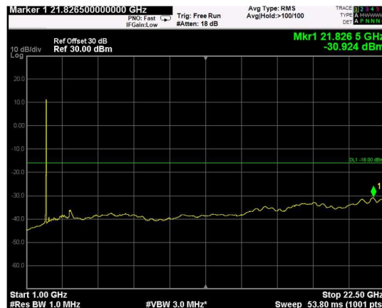
Channel: BOTTOM, Modulation: QPSK, BW=5MHz, Range: Upper
