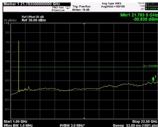
Channel: TOP, Modulation: 16QAM, BW=15MHz, Range: Upper
