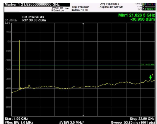
Channel: TOP, Modulation: 16QAM, BW=5MHz, Range: Upper
