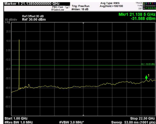
Channel: MIDDLE, Modulation: 64QAM, BW=15MHz, Range: Upper
