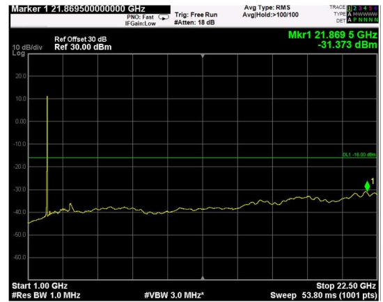
Channel: BOTTOM, Modulation: 64QAM, BW=10MHz, Range: Upper
