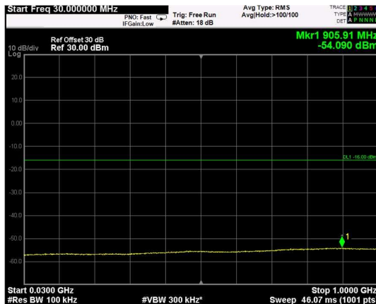
Channel: MIDDLE, Modulation: 64QAM, BW=15MHz, Range: Lower
