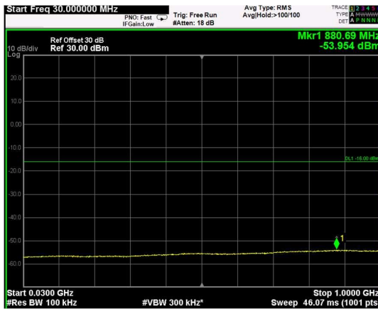
Channel: BOTTOM, Modulation: 16QAM, BW=5MHz, Range: Lower
