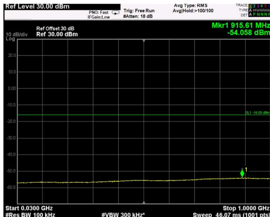
Channel: MIDDLE, Modulation: 256QAM, BW=15MHz, Range: Lower
