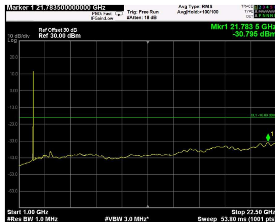
Channel: BOTTOM, Modulation: 256QAM, BW=5MHz, Range: Upper
