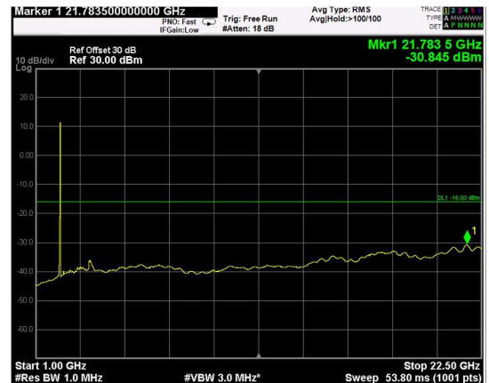
Channel: MIDDLE, Modulation: 256QAM, BW=10MHz, Range: Upper
