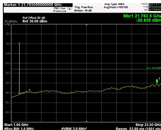
Channel: TOP, Modulation: 256QAM, BW=5MHz, Range: Upper
