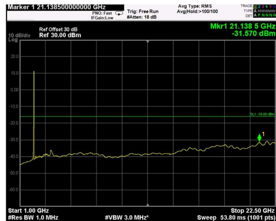
Channel: TOP, Modulation: QPSK, BW=15MHz, Range: Upper
