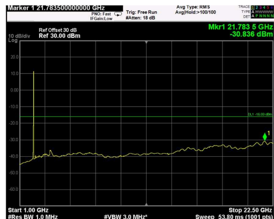
Channel: TOP, Modulation: 64QAM, BW=15MHz, Range: Upper
