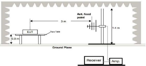
(3) Radiated Emission Test-Up Frequency Above 1GHz
