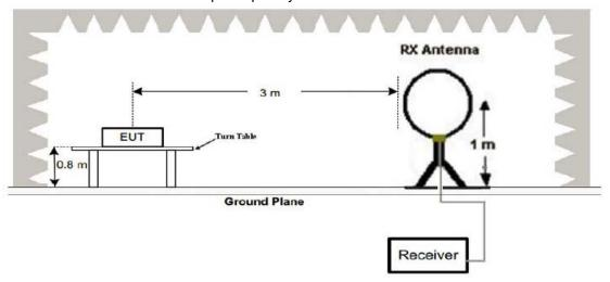
(2) Radiated Emission Test-Up Frequency 30MHz~1GHz
