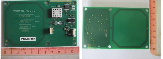
In the field BBNR2 the FCC ID is printed, it reads "FCC ID: HPL-DSRFID-D". In the field BBNR1 the Agfa article code is printed, it reads "A800126.XX" where XX is the PCB assembly version index 07 or larger. In the field SNR1 the PCB assembly serial number is printed. The prototype used for the radio type testing is s/n RS2408059001.
