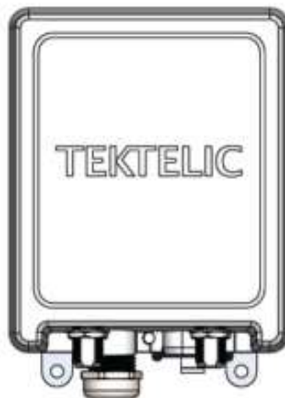
Figure 6: Kona Enterprise Gateway Module Wall Mounting Orientation
