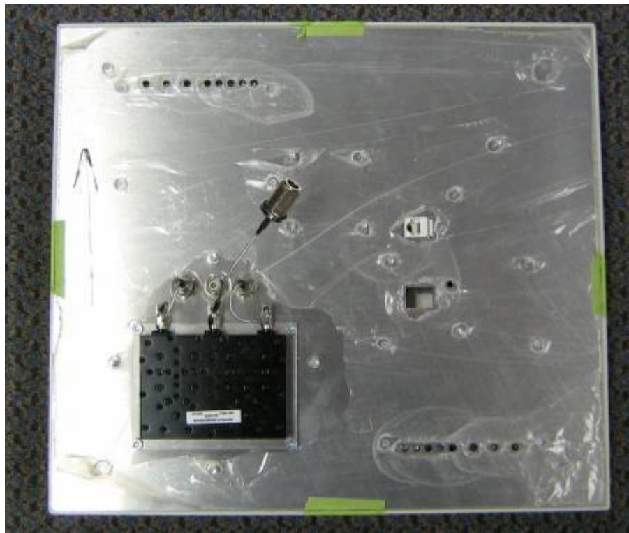
The N connector used for external antennas
