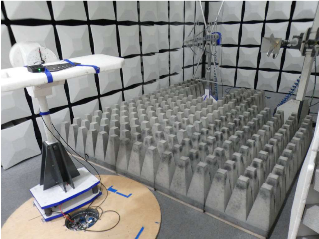
Photo 3: Setup Spurious Emissions Radiated (FAC), > 1GHz
