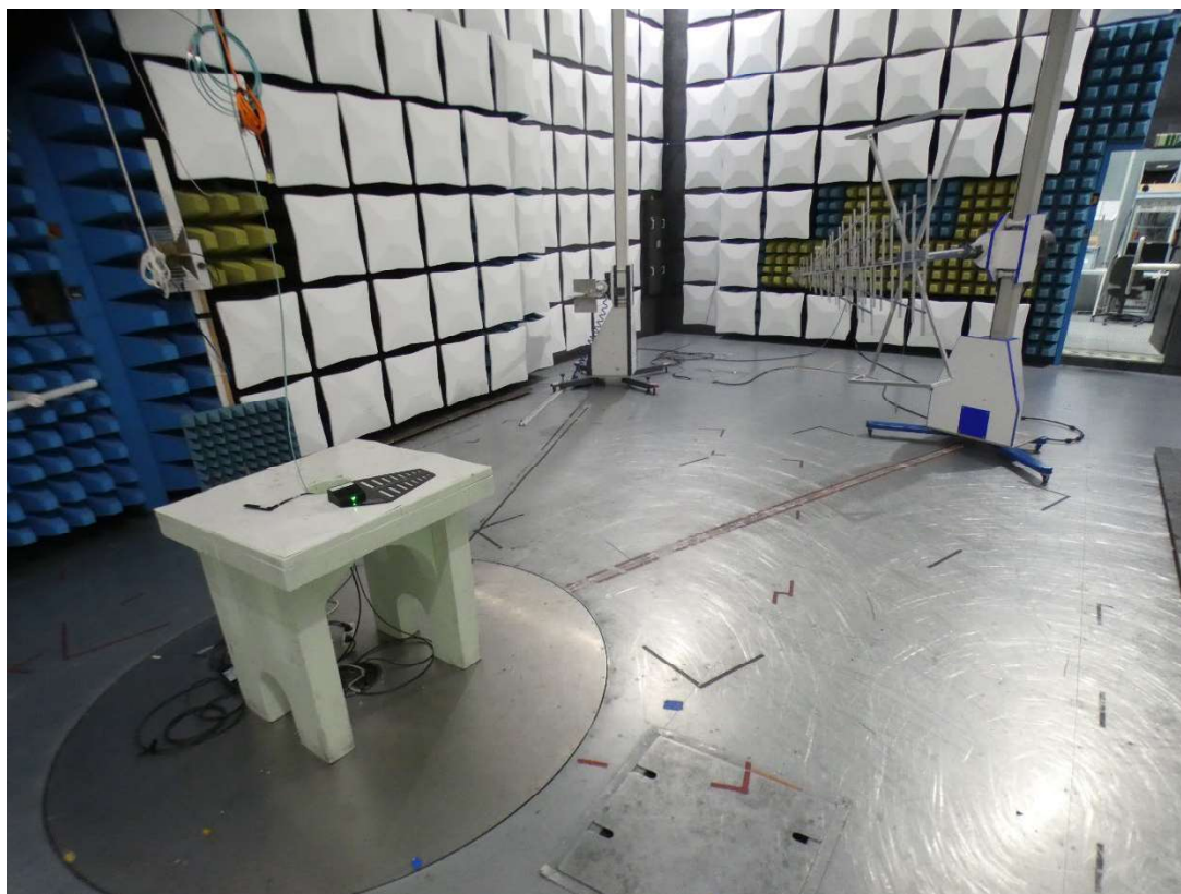
Photo 1: Setup Spurious Emissions Radiated (SAC), < 1 GHz
