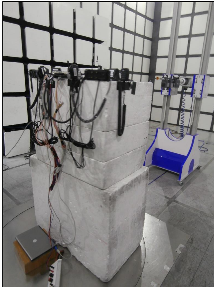
Figure 33 - Test Setup – 18 GHz to 25 GHz (Middle View) – X Orientation
