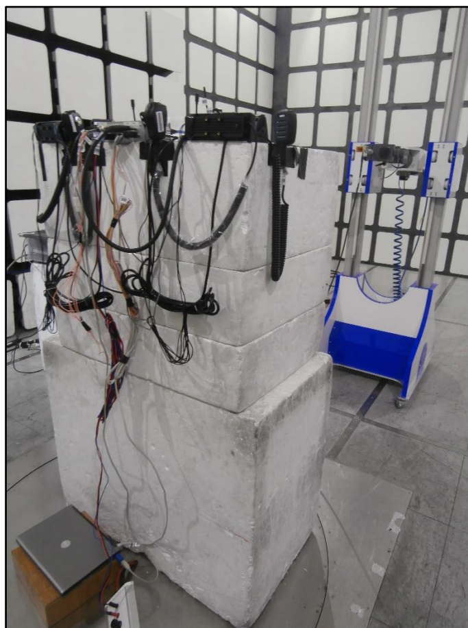
Figure 32 - Test Setup – 18 GHz to 25 GHz (Left View) – X Orientation
