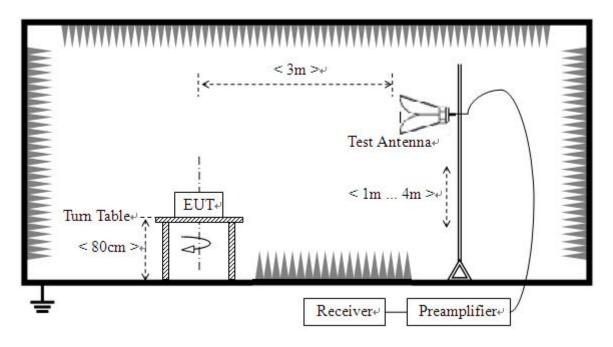
(For Radiated Emission Test (above 1 GHz))
