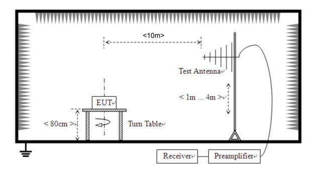
(For Radiated Emission Test (30 MHz-1 GHz))
