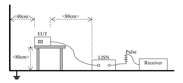
(For Conducted Emission, AC Ports Test)
