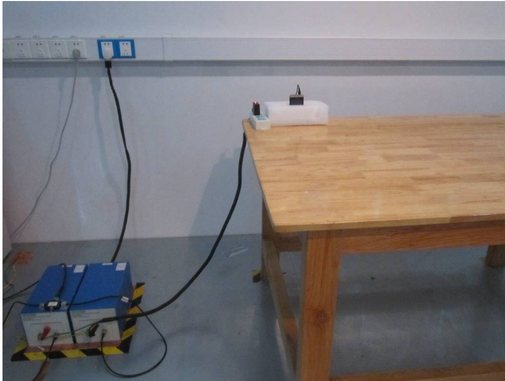
Conducted Emissions Test Setup Front View
