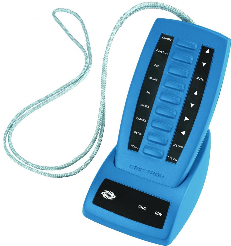
WPR-48 Waterproof Wireless Handheld Remote with Lanyard and Customized Button Labels, Mounted in Docking Station
