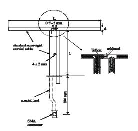
APREL Laboratories have developed frequency dipoles based on current scientific research carried both experimentally numerically here at the APREL Laboratories site. Mechanical and electrical parameters for the dipoles established have been experimental and numerical techniques, and target SAR values have been established following IEC methodologies. The results of the experimental and numerical research have been published and released for peer review.
