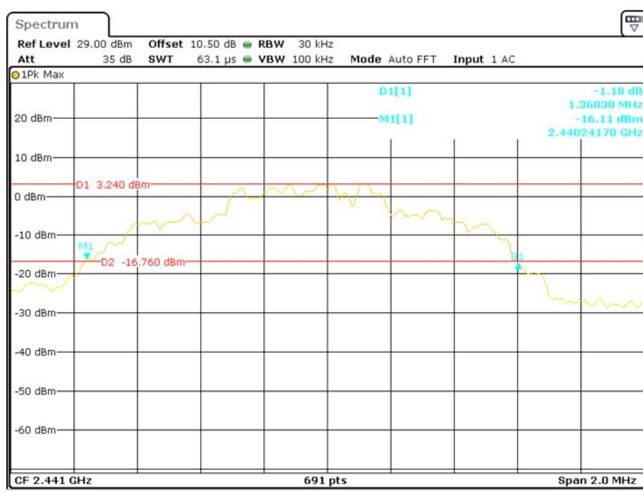
**EDR ( $\pi/4$ -DQPSK): High Channel**
