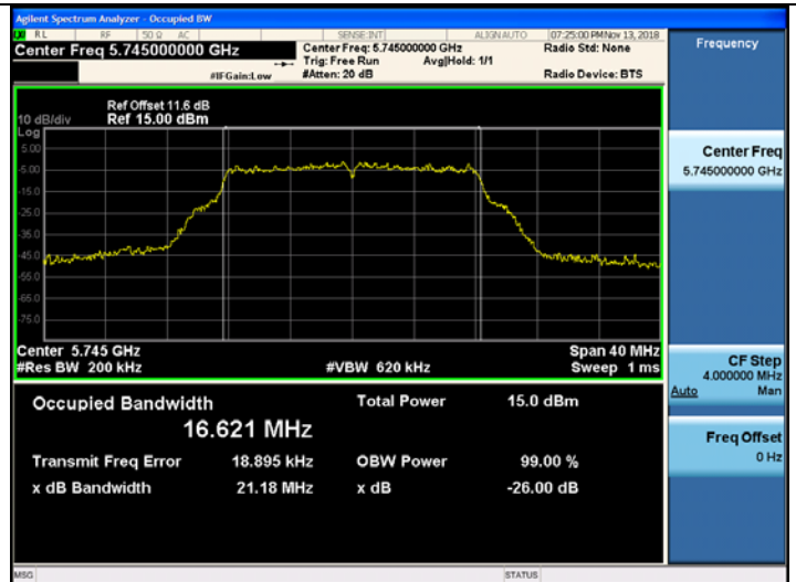
802.11a UNII 3 BAND 26dB Bandwidth (CH 149)
