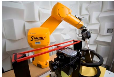
Figure 4-3 SPEAG Robotic System
