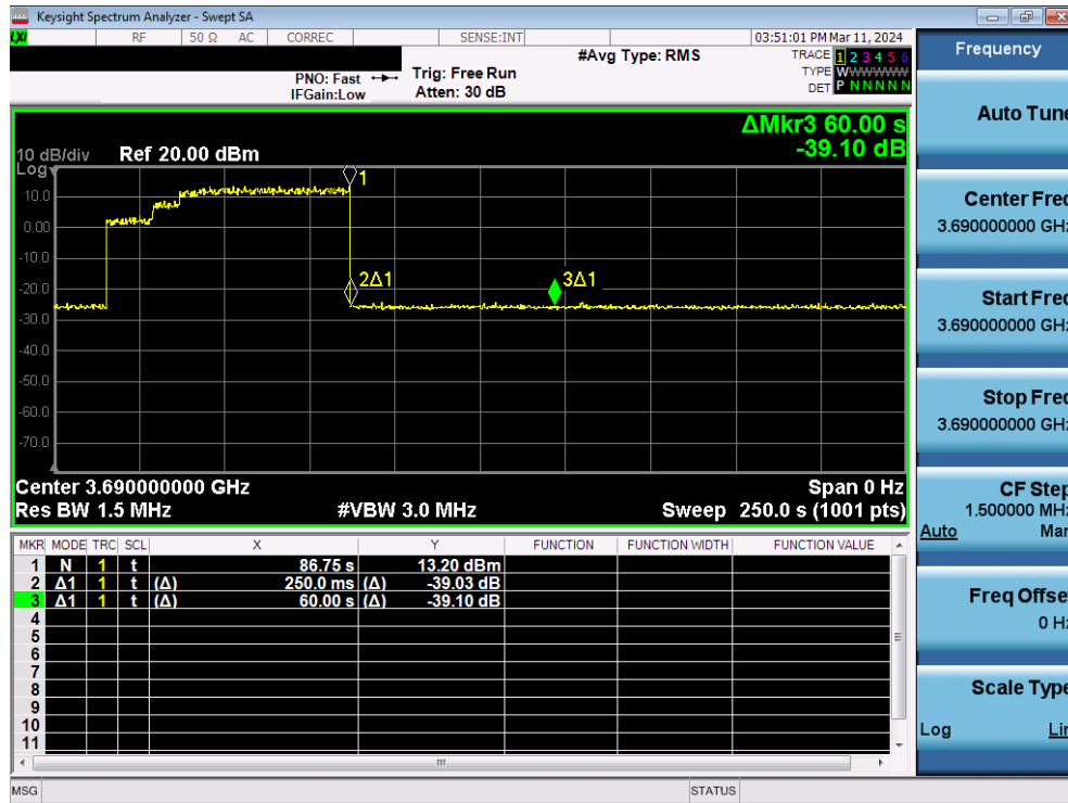
Plot 18. Conducted Measurement – RF transmission stops within 60s of SAS RLQ response (Marker 1) (WINNF.FT.C.RLQ.1)
