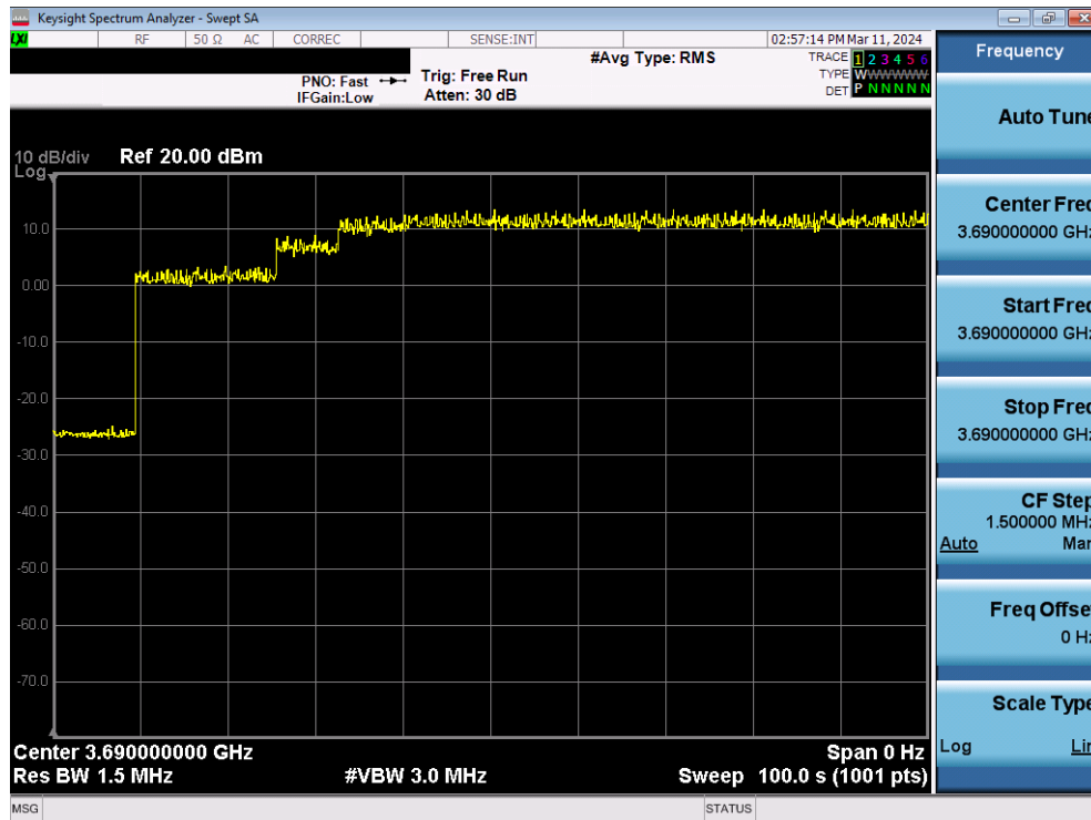
Plot 10. Conducted Measurement - RF transmission after SAS heartbeat response (WINNF.FT.C.HBT.1)
