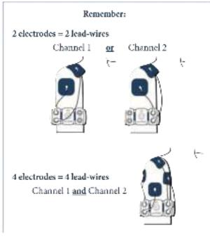
• **Step 1**: clip the narrow end of the cables to either 2 or 4 electrodes.
