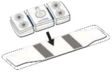
• **Step 4**: stick the self-adhesive strip attached to the actiTENS near to the electrodes.
