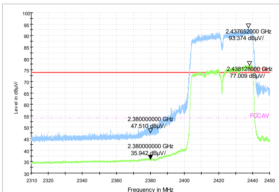
Fig.127 Frequency Band Edge: Ch3,11n(40M)
