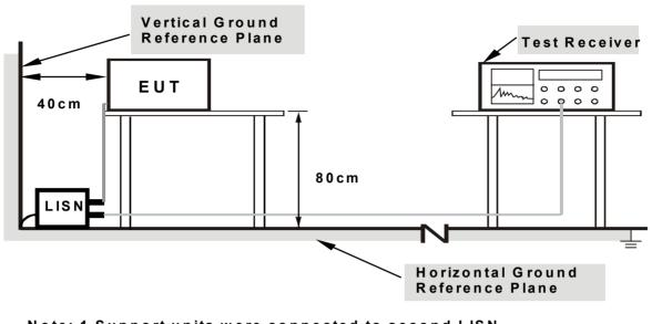
Note: 1.Support units were connected to second LISN. 2.Both of LISNs (AMN) are 80cm from EUT and at least 80cm from other units and other metal planes support units.
