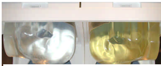
Figure 7.1 Left and Right SAM Phantom shells
