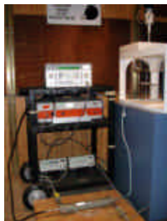
Figure A.0 Dipole Validation Test Setup
