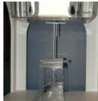
Figure A.0 Dipole Validation Test Setup
