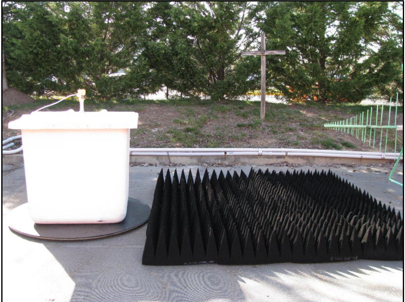
Photograph 66: Radiated Emissions – TC #9; Fiberglass Container, Rear View
