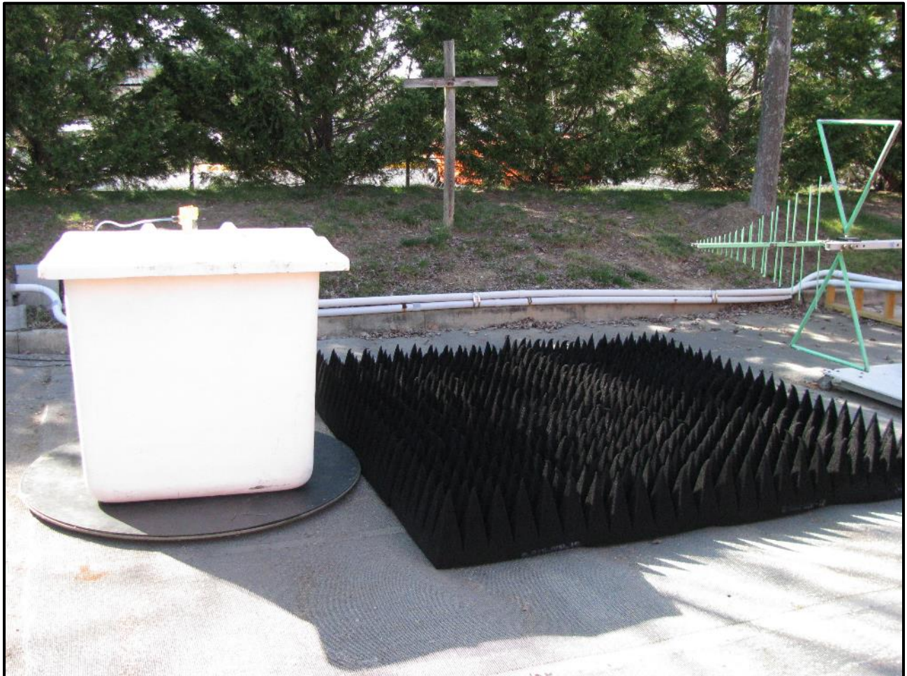
Photograph 56: Radiated Emissions – TC #4; Fiberglass Container, Rear View
